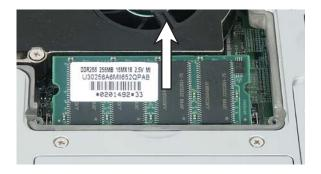
**8** Hold the new or replacement module at a 30-degree angle and press it into the empty memory slot. This module is keyed so it can only be inserted in one direction. If the module does not fit, make sure that the notch in the module lines up with the tab in the memory bay.
