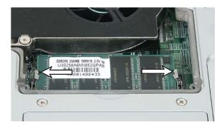
**7** Pull the memory module out of the slot.
