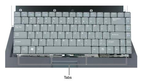
**3** Gently press the keyboard down until it is flat all the way across. The keyboard should easily fall into place. Be careful not to damage the LCD panel.
